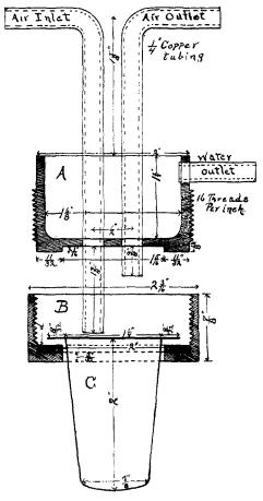
flange, or the flange of the crucible may rest directly upon the casing flange and the washer placed on top of the crucible flange. The author has used a pure rubber washer, letting it rest directly upon the flange of the crucible, which in turn rested upon the casing flange of B, but it was found that the blank determinations were always high, that is 0.0008 gram, but were constant, if care
